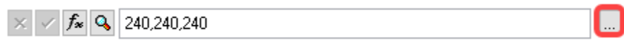
Figure 14. Use the ellipsis button in the Property Sheet to access a property editor. Double-clicking the property or its value does the same thing.
